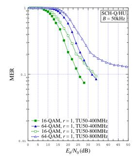
Figure 9.59: MER vs.  $E_b / N_0$  for B = 50 kHz, SCH-Q/HU, TU50-400 MHz and TU50-800 MHz channels, 16-QAM r = 1 and 64-QAM r = 1
