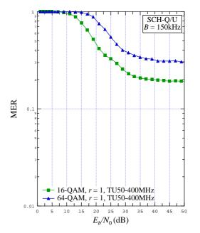
Figure 9.73: MER vs.  $E_b/N_0$  for B = 150 kHz, SCH-Q/U, TU50-400 MHz channel, 16-QAM r = 1 and 64-QAM r = 1
