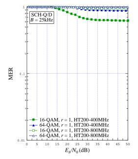
Figure 9.50: MER vs.  $E_b / N_0$  for B = 25 kHz , SCH-Q/D, HT200-400 MHz and HT200-800 MHz channels, 16-QAM r = 1 and 64-QAM r = 1
