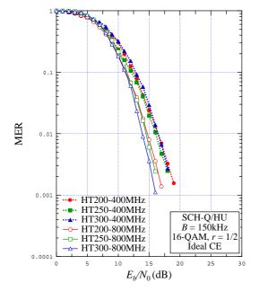
Figure C.3: MER vs.  $E_b / N_0$  for B = 150 kHz, SCH-Q/HU, 16-QAM r = 1/2, various HT channels and ideal CE
