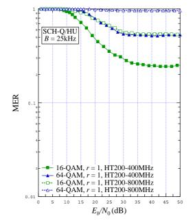
Figure 9.62: MER vs.  $E_b / N_0$  for B = 25 kHz , SCH-Q/HU, HT200-400 MHz and HT200-800 MHz channels, 16-QAM r = 1 and 64-QAM r = 1
