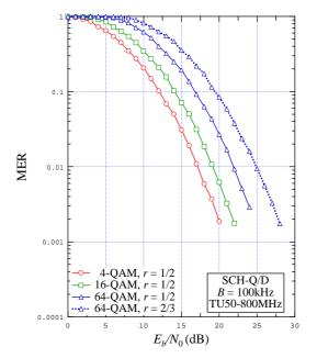
Figure 9.11: MER vs.  $E_b / N_0$  for B = 100 kHz, SCH-Q/D, TU50-800 MHz channel, various modulations/coding rate combinations
