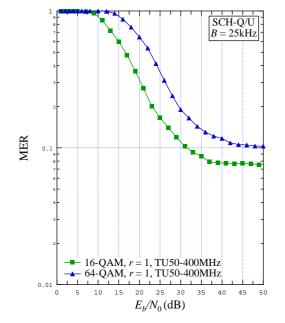
Figure 9.70: MER vs.  $E_b/N_0$  for B = 25 kHz , SCH-Q/U, TU50-400 MHz channel, 16-QAM r = 1 and 64-QAM r = 1
