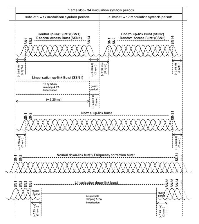
Figure 6.4: Burst types for QAM
