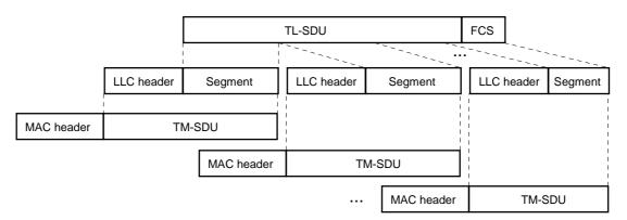
Figure 7.8: Advanced link segmentation by the LLC
