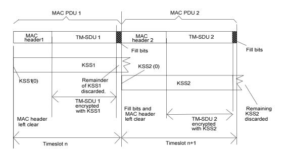
Figure 13.2: Fixed-mapped allocation of KSS to encrypt QAM MAC PDUs
