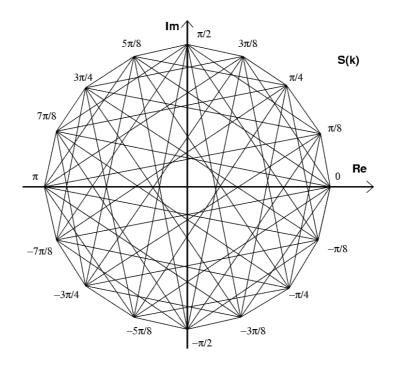
Figure 6.9:  $\pi$ /8-D8PSK modulation symbol constellation and possible transitions
