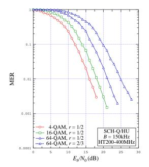
Figure 9.28: MER vs.  $E_b / N_0$  for B = 150 kHz, SCH-Q/HU, HT200-400 MHz channel, various modulations/coding rate combinations
