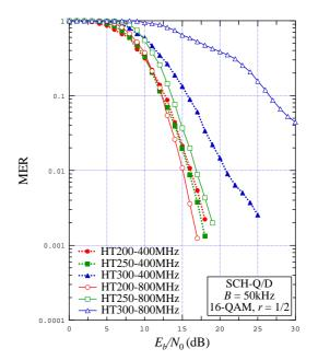
Figure 8.3: MER vs.  $E_b / N_0$  for B = 50 kHz , SCH-Q/D, 16-QAM r = 1/2 , various HT channels
