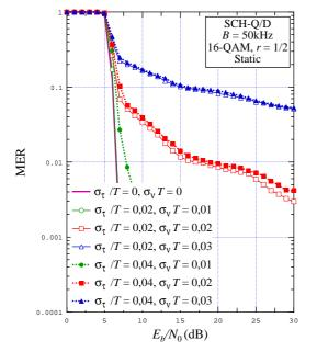
Figure 6.20: MER vs.  $E_b/N_0$  for B = 50 kHz, SCH-Q/D, 16-QAM r = 1/2, static channel, various combinations of timing and frequency synch. errors
