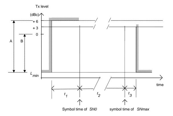
A: Mask height specified for phase modulation.
