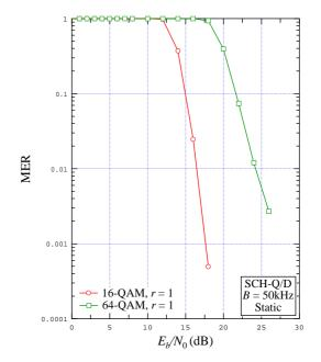
Figure 9.55: MER vs.  $E_b / N_0$  for B = 50 kHz , SCH-Q/D, static channel, 16-QAM r = 1 and 64-QAM r = 1
