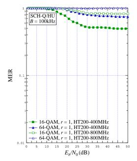
Figure 9.64: MER vs.  $E_b / N_0$  for B = 100 kHz , SCH-Q/HU, HT200-400 MHz and HT200-800 MHz channels, 16-QAM r = 1 and 64-QAM r = 1
