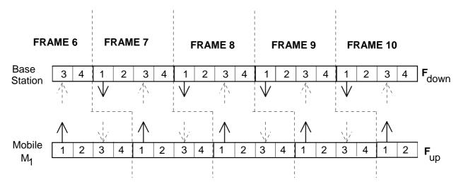
Figure 7.5: Uplink and downlink slot and TDMA frame arrangements
