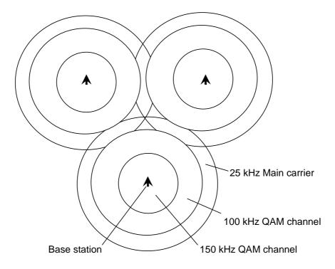
Figure 7.18: Example of cells using non-conforming concentric channels
