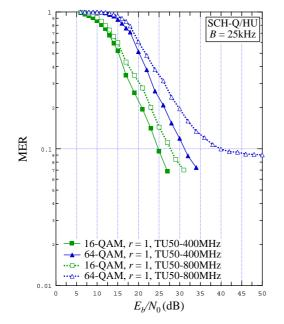
Figure 9.58: MER vs.  $E_b / N_0$  for B = 25 kHz, SCH-Q/HU, TU50-400 MHz and TU50-800 MHz channels, 16-QAM r = 1 and 64-QAM r = 1
