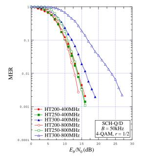
Figure 8.2: MER vs.  $E_b / N_0$  for B = 50 kHz, SCH-Q/D, 4-QAM r = 1/2, various HT channels
