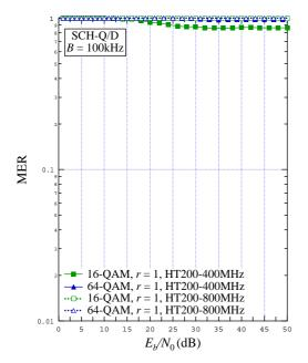
Figure 9.52: MER vs.  $E_b / N_0$  for B = 100 kHz, SCH-Q/D, HT200-400 MHz and HT200-800 MHz channels, 16-QAM r = 1 and 64-QAM r = 1
