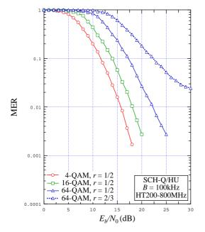
Figure 9.35: MER vs.  $E_b / N_0$  for B = 100 kHz , SCH-Q/HU, HT200-800 MHz channel, various modulations/coding rate combinations
