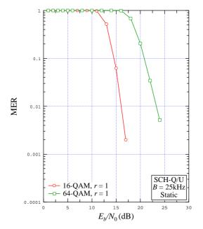
Figure 9.74: MER vs.  $E_b / N_0$  for B = 25 kHz, SCH-Q/U, static channel, 16-QAM r = 1 and 64-QAM r = 1
