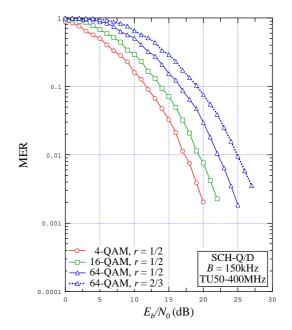
Figure 9.4: MER vs.  $E_b/N_0$  for B = 150 kHz, SCH-Q/D, TU50-400 MHz channel, various modulations/coding rate combinations
