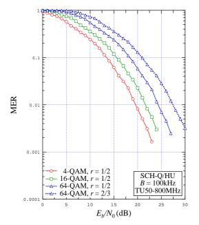
Figure 9.31: MER vs.  $E_b / N_0$  for B = 100 kHz , SCH-Q/HU, TU50-800 MHz channel, various modulations/coding rate combinations
