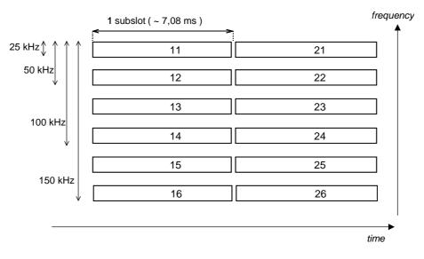
Figure 7.16: Random access time / frequency structure for QAM channels
