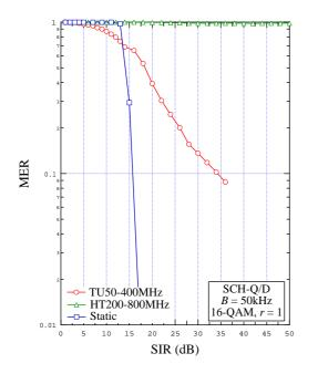
Figure 9.78: MER vs. SIR for B = 50 kHz, SCH-Q/D, 16-QAM r = 1, various channel combinations
