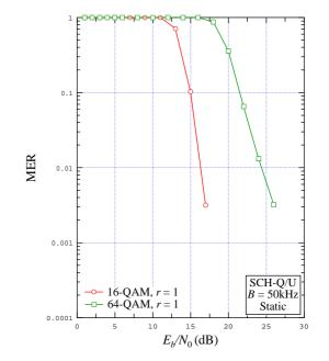
Figure 9.75: MER vs.  $E_b / N_0$  for B = 50 kHz, SCH-Q/U, static channel, 16-QAM r = 1 and 64-QAM r = 1
