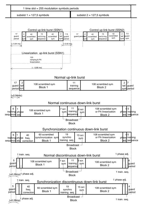
Figure 6.3: Burst types for phase modulation
