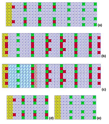
Figure 6.5: Structure of NUB (a), NDB (b), FCB (c), CB (d) and RAB (e), for a 25 kHz (8 sub-carrier) QAM channel
