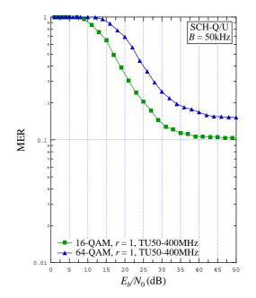
Figure 9.71: MER vs.  $E_b / N_0$  for B = 50 kHz, SCH-Q/U, TU50-400 MHz channel, 16-QAM r = 1and 64-QAM r = 1
