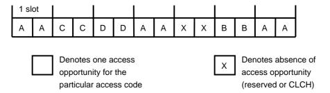
Figure 7.13: Example of subslot structure on assigned SCCH
