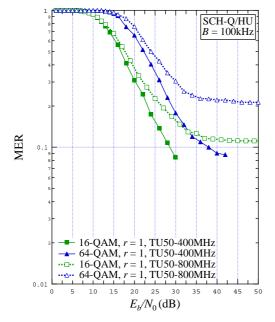
Figure 9.60: MER vs.  $E_b / N_0$  for B = 100 kHz, SCH-Q/HU, TU50-400 MHz and TU50-800 MHz channels, 16-QAM r = 1 and 64-QAM r = 1
