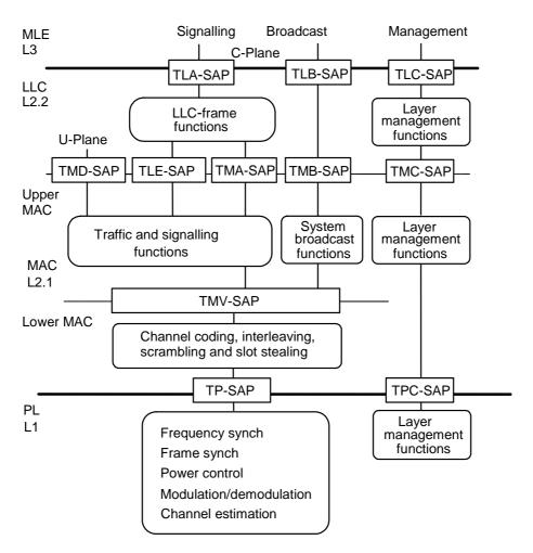
Figure 7.4: Layer 2 reference architecture
