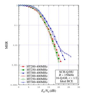
Figure C.4: MER vs.  $E_b/N_0$  for B = 150 kHz, SCH-Q/HU, 16-QAM r = 1/2, various HT channels and ideal BCE
