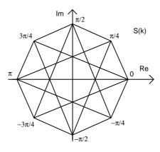
Figure 6.8: π/4-DQPSK modulation symbol constellation and possible transitions
