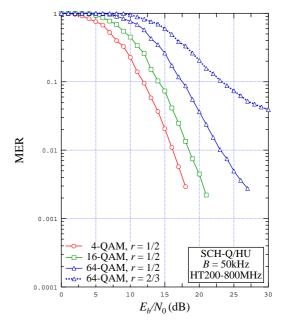
Figure 9.34: MER vs.  $E_b / N_0$  for B = 50 kHz, SCH-Q/HU, HT200-800 MHz channel, various modulations/coding rate combinations
