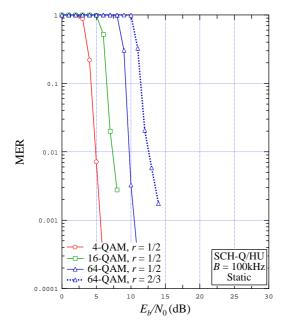
Figure 9.39: MER vs.  $E_b / N_0$  for B = 100 kHz , SCH-Q/HU, static channel, various modulations/coding rate combinations
