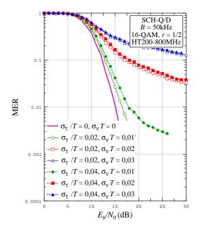
Figure 6.19: MER vs.  $E_b / N_0$  for B = 50 kHz , SCH-Q/D, 16-QAM r = 1/2 , HT200-800 MHz channel, various combinations of timing and frequency synch. errors
