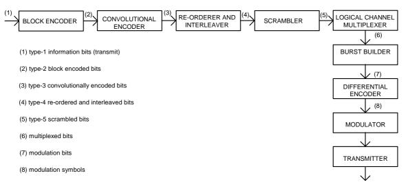
Figure 6.6: Reference configuration for phase modulation
