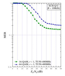
Figure 9.72: MER vs.  $E_b / N_0$  for B = 100 kHz , SCH-Q/U, TU50-400 MHz channel, 16-QAM r = 1and 64-QAM r = 1
