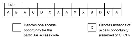
Figure 7.12: Example of subslot structure on common control channel
