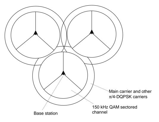
Figure 7.19: Example of CA cells using sectored channels
