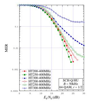
Figure 8.7: MER vs.  $E_b / N_0$  for B = 50 kHz, SCH-Q/HU, 64-QAM r = 1/2, various HT channels
