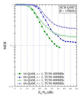
Figure 9.61: MER vs.  $E_b/N_0$  for B = 150 kHz , SCH-Q/HU, TU50-400 MHz and TU50-800 MHz channels, 16-QAM r = 1 and 64-QAM r = 1
