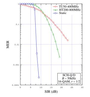
Figure 9.44: MER vs. SIR for B = 50 kHz, SCH-Q/D, 16-QAM r = 1/2, various channel combinations
