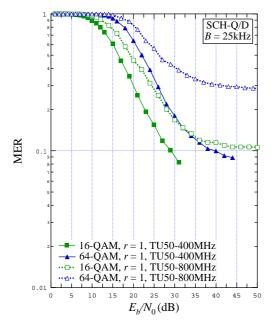
Figure 9.46: MER vs.  $E_b / N_0$  for B = 25 kHz, SCH-Q/D, TU50-400 MHz and TU50-800 MHz channels, 16-QAM r = 1 and 64-QAM r = 1
