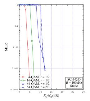
Figure 9.19: MER vs.  $E_b / N_0$  for B = 100 kHz, SCH-Q/D, static channel, various modulations/coding rate combinations
